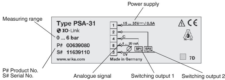
If the serial number becomes illegible (e.g. due to mechanical damage or overpainting), traceability will no longer be possible.
